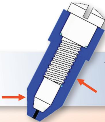
*The improved valve design found in the commercial line of buoys and fenders incorporates a newly designed seating surface and increased thread length to prevent leakage and to help prevent strip-out.*
